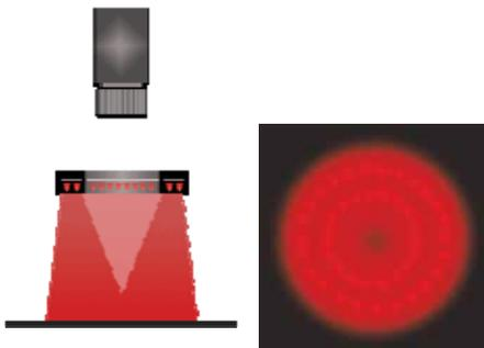
Fig. 20a – Bright field image of a mirror.
