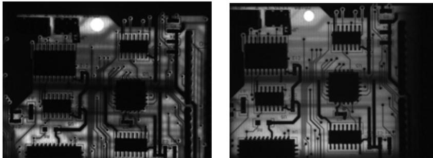
Fig 13 – Populated PCB. Penetration of red 660 nm (left image) and IR 880 nm light. Notice the better penetration of IR despite the red blooming out from the hole in the top center of the board.
