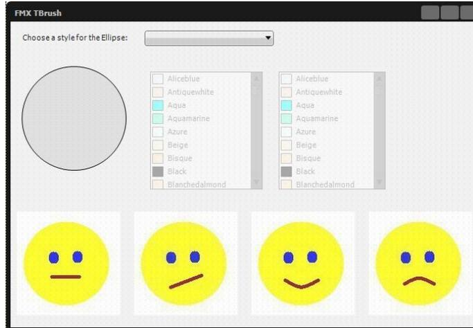
Disable all the components, except the Ellipse, the ComboBox, and the Labels. Set the text to the labels as null (''), except for the one above the ComboBox. Set its text to 'Choose a style for the Ellipse:'. Load different Bitmap files to the Bitmap property of the Image objects.
